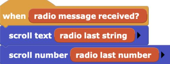
You can also send numbers as “codes” from one micro:bit to trigger actions on another. For example, send a “1” to show an LED matrix pattern, and a “0” to clear it. The sender acts like a remote control.
